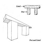
The Parthenon was built using post-and-lintel construction.
